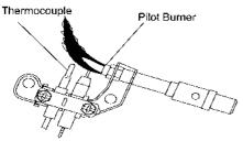
Figure 14 - Incorrect Pilot Flame Pattern
